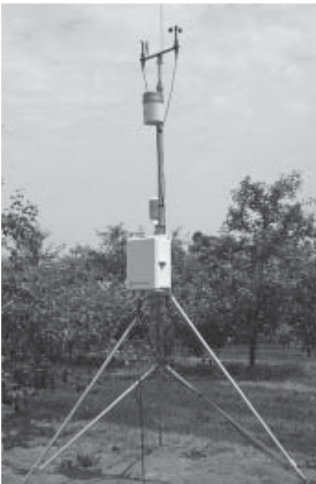
Figure 1. Weather stations are used to monitor maximum and minimum temperature and wetting periods from rain and dew. The data are entered into a disease prediction model to time streptomycin application to control blossom blight, and to predict symptom development for all phases of the disease.
